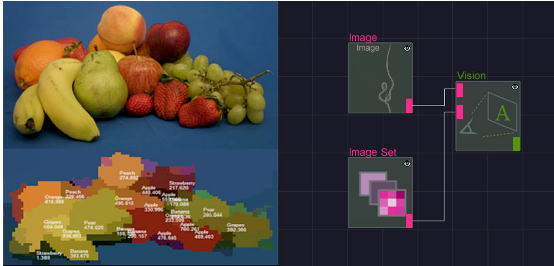
Figure 6.22: Computer vision in LUNA with two inputs, 1) an image set representing a memory of objects, fruits from various angles and 2) a target image of a still life to be detected (top left), produces a set of labelled points (bottom left) of detected objects.
