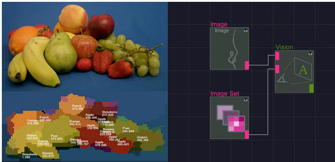
Figure 6.23: Computer vision in LUNA with two inputs, 1) an image set representing a memory of objects, fruits from various angles and 2) a target image of a still life to be detected (top left), produces a set of labeled points (bottom left) of detected objects.
